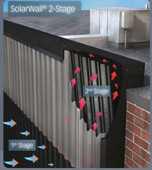
1st Stage - Sun heats SolarWall® collector and fresh air is heated as it passes through the surface
