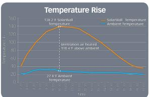
Data from Plattsburgh Intl Airport - February 4, 2012 Avg SW 2-Stage performance data when horizontal solar radiation exceeds 300 W/m<sup>2</sup>
